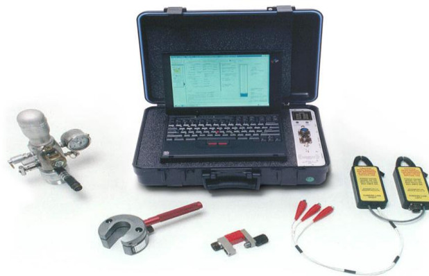
Figura 2 - Equipamento total well management (Echometer Company, 2005)
